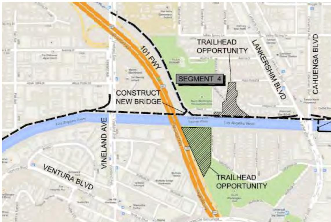
The preferred alternative alignment for the bike path between the 101 Freeway and Lankershim Blvd. is on the north side of the LA River. This alternative is considered the best option because of difficulties accessing the road at grade at Lankershim Blvd, given the narrow available right of way east of Lankershim Blvd.
